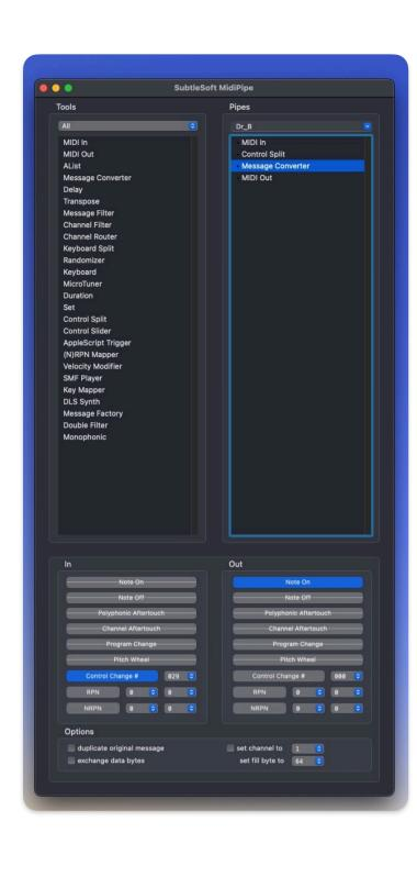
One of two MIDI pipes; the CC29 message gets converted to note on messages; yes plural! the magic that makes this routine so effective is that both CC29 messages (127 AND 0) get converted into note on values; in effect that means stepping and releasing each effectively drive the GP script in essence only using one note, this is a fluke I'll admit I stumbled on it literally, 'step-pled' on it actually
